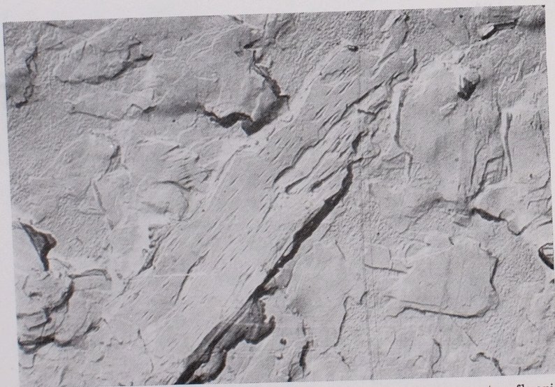
Phot. 8. Electron micrograph (replica technique) of kaolinite aggregates fluorinated with 2 n \text{NH}_4\text{F} solution for 8 hours. Magn. \times 16,000
