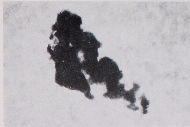
Phot. 5. Electron micrograph of a single kaolinite flake after 15-hour fluorination with 1.5 n \text{NH}_4\text{F} solution. Magn. \times 17,000
