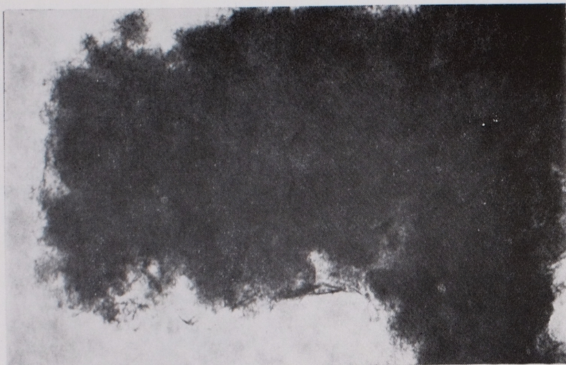
Phot. 3. Electron micrograph of kaolinite aggregate after 5-hour fluorination with 1.5 n \text{NH}_4\text{F} solution. Magn. \times 15,000
