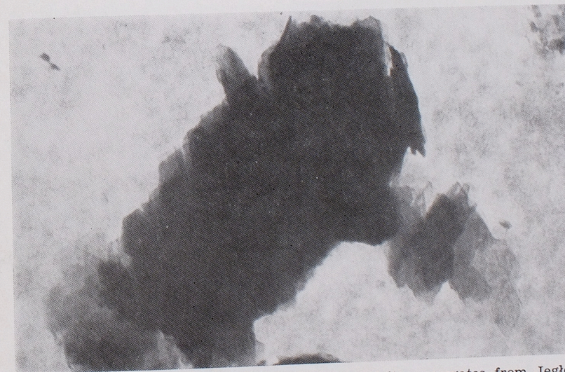
Phot. 2. Electron micrograph of polycrystalline kaolinite aggregates from Jegłowa before fluorination. Magn. \times 32,000
